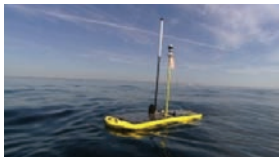
The Wave Glider is a floating sensor that tracks marine life and monitors ocean chemistry. This solar-powered aquatic drone's unlimited range allows it to survey marine life in the ocean's depths for months at a time, relaying its findings back to Dalhousie via satellite in real time.
